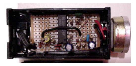
Here is how I tested the circuit. The RCX has a Visual Basic program that produces a 15kHz tone and watches the input for levels over 33. If is sees one, it turns on an output which just has a light hooked up to it. The operating range depends on many mechanical factors. It can pickup motion of large objects 8" away while small objects may need to be only a few inches between the RCX and the microphone.
